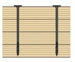
screw: TBSF8149 timber element: 4 x 1 1/2" (38 mm) total thickness: 6" (152 mm)
